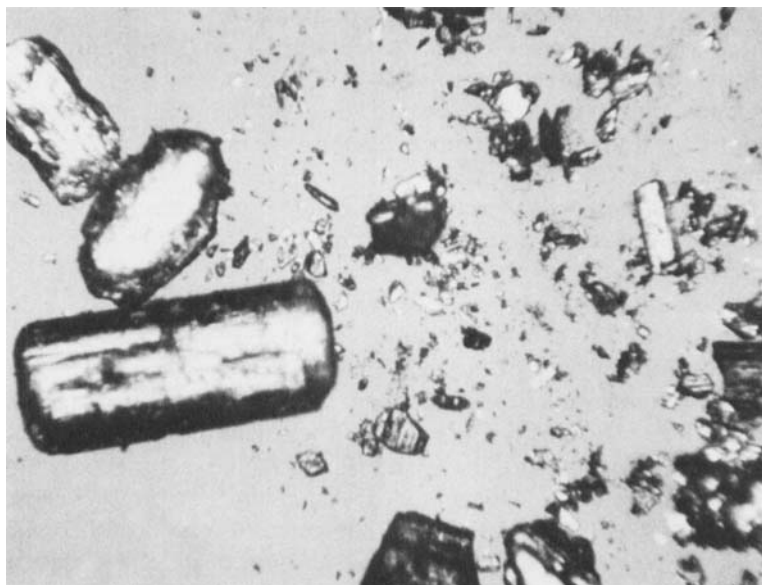
FIGURE 5 Optical micrograph of virgin OPCTS. The largest crystallites are \approx 1000 \mu\text{m} in length, the smallest \approx 50 \mu\text{m} . From the micrograph we see that it is reasonable to approximate the crystallite size distribution as bimodal (a few large ones, many small ones).
